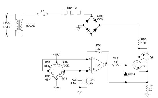
Figure 5-5. Detector Heater Control Circuit
